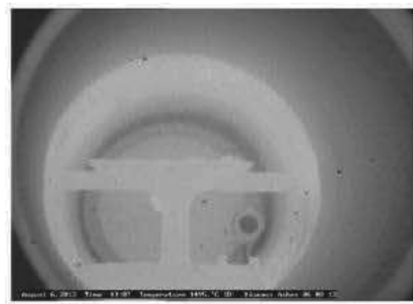
Fig. 10: Ash fusion Test Result for Coal Ash Sample (Fluid Temperature)
