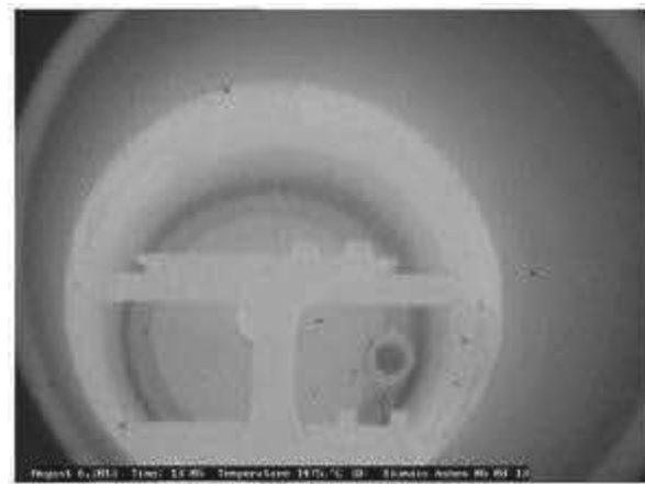
Fig. 8: Ash Fusion Test Result for Coal Ash Sample (Softening Temperature)
