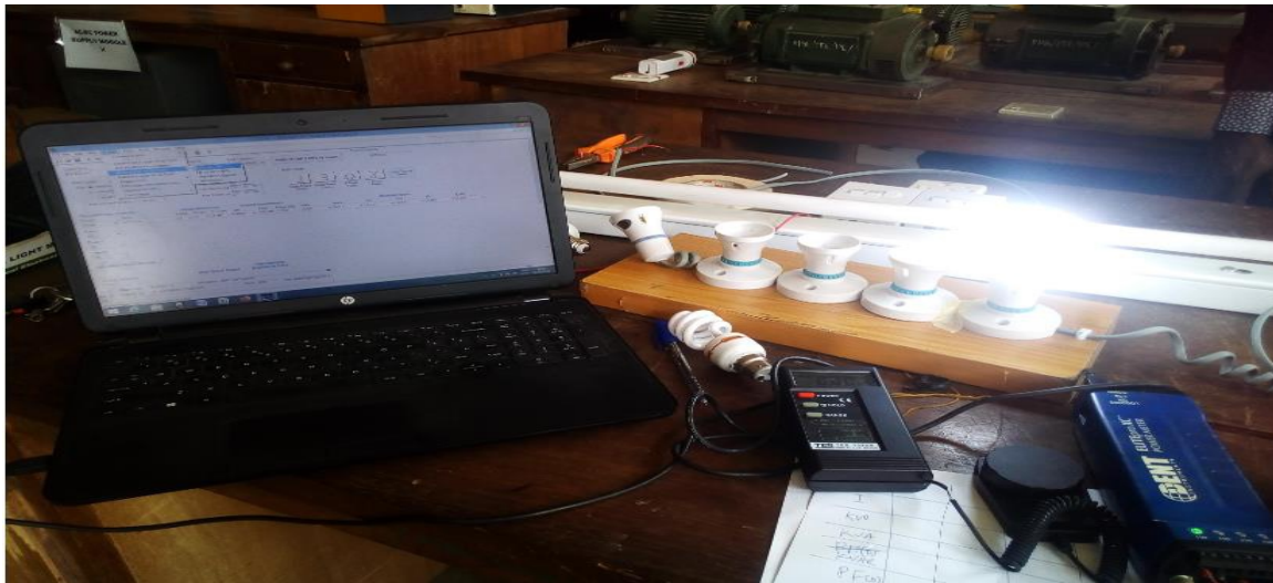
Figure : Experimental setup for power quality measurement with DENT Power logger
