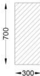
Fig 6: 2D Geometry of Rectangular Concrete Beam Dimension
