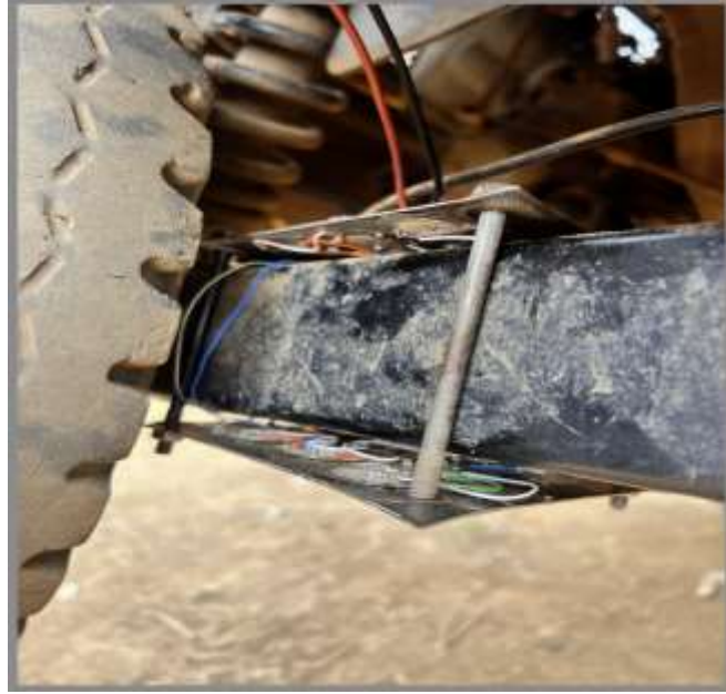
Plate 2: The tricycle suspension system fitted with the energy harvester
