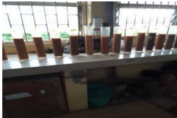
Plate 2: The graduated cylinder setup for particle soil analysis
