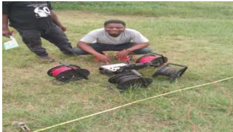
Plate 1: Electrical resistance measurement setup
