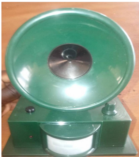
Fig. 4: Bird Repeller used for the system
