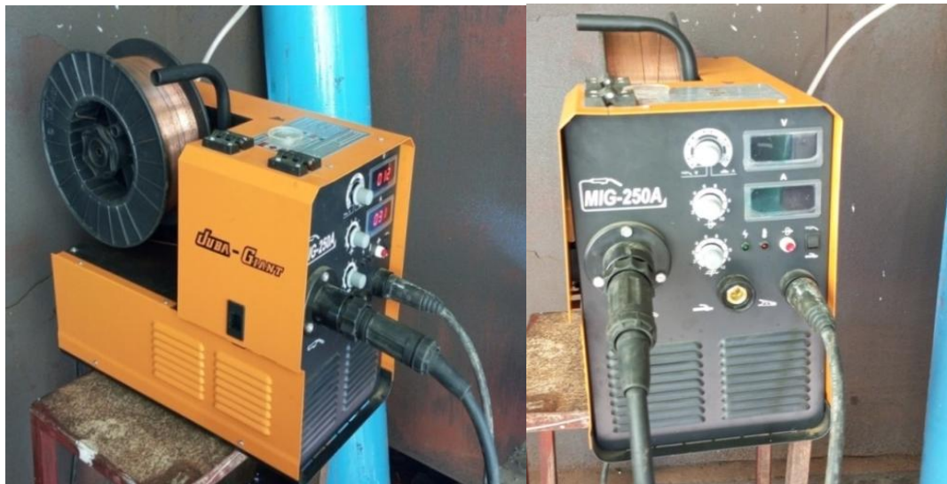
Figure 2: JUBA GIANT MIG-250A (GMAW Machine (left) and the settings (right)
