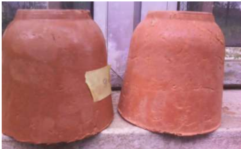
Fig 13: Crucible Produced at Pressure of 90 bar and Sieve Size 0.6 and 1.70 mm respectively
