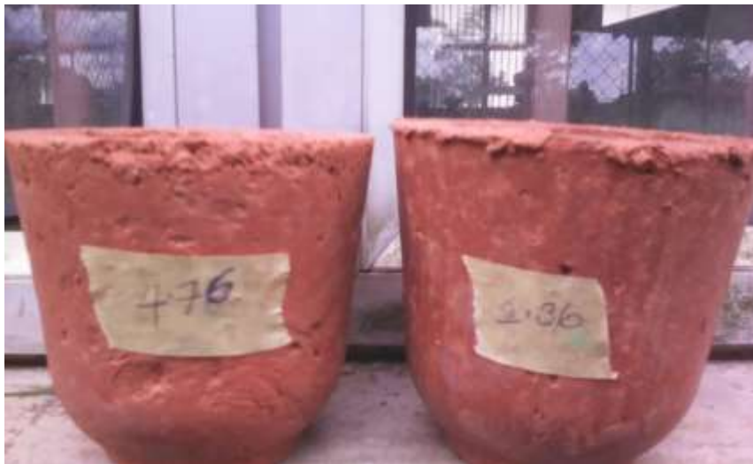
Fig 14: Crucible Produced at Pressure of 100 bar and Sieve Size 4.76 and 2.36 mm respectively
